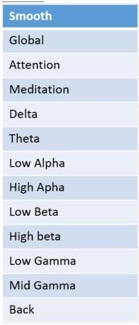
The "smooth" is a sort of low pass filter that we apply on the data coming from the headset. Neurosky MindwaveMobile calculates the EEG power spectrum and the Attention and Meditation values each second. A value of 0 does not smooth at all the outputs (either the DAC outputs and the MIDI values) and a value of 100 helds a time constant of about 2 seconds. We suggest to use 95 for an 'organic' trend of the outputs.
